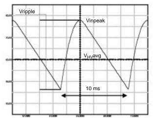
Figure 7b. A Typical Ripple Voltage over the Bulk Capacitor
