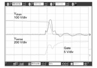
Figure 11c. This shot confirms our turn-on 45 ns calculation and shows the absence of immediate drain current. The capacitive peak is blanked with the NCP1200 LEB.
