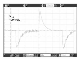
Figure 11f. Demoboard transient response when banged from 10 mA to 800 mA.
