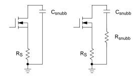
Figure 6b. If the output power is low, you can wire a simple capacitor MOSFET's drain and ground.
