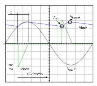
Figure 8a. When V<sub>AC</sub>in reaches Vpeak, the diode stops conducting.
