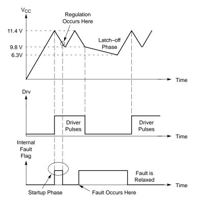
Figure 5. If the fault is relaxed during the V<sub>CC</sub> natural fall down sequence, the IC automatically resumes. If the fault still persists when V<sub>CC</sub> reached UVLO<sub>L</sub>, then the controller enters burst mode until recovery.
