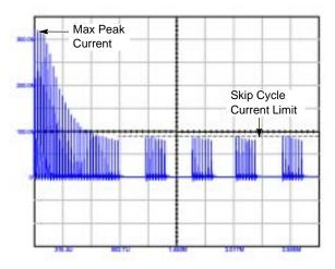
Figure 4c. The skip cycle takes place at low peak currents which guarantees noise–free operation.
