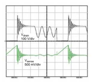
Figure 10b. Steady–State Drain–Source and Sense Voltages
