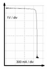
Figure 12f. The Resulting I–V Curve of the NCP1200 Charger Demoboard
