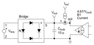
Figure 7a. A Full–Wave Rectification Configuration
