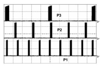
Figure 4b. Output pulses at various power levels  $(X = 5 \ \mu s/div) P3 < P2 < P1$
