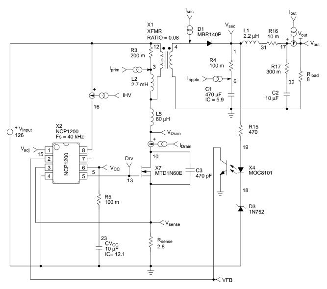
Figure 10a. A typical transient analysis of the NCP1200 with a dedicated SPICE model. C3 is purposely wired between drain–source to highlight the potential substrate injection problems.
