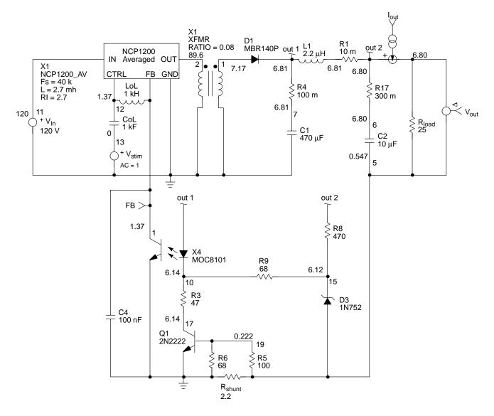
Figure 12a. An Averaged SPICE Simulation in a Battery Charger Application
