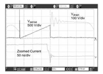
Figure 11e. Wiring the snubber between drain and source avoids the substrate injection.
