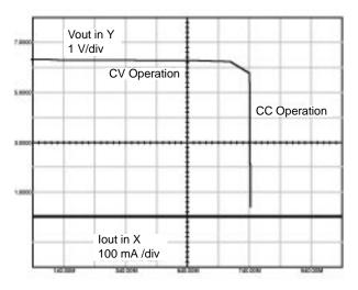
Figure 12d. The simulated CC–CV output shape as delivered by Figure 12a.
