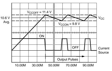
Figure 1b. DSS Waveforms During Start–Up and Normal Mode ( $CV_{CC}$  = 10  $\mu$ F)
