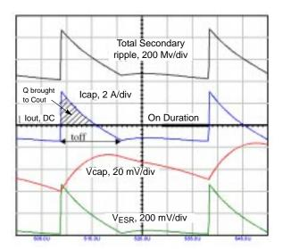
Figure 9b. The final ripple is made of the ESR and the output capacitance.
